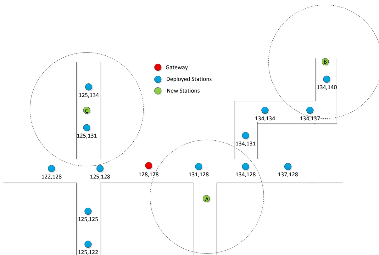
Figure 1: Typical Address Configuration with Both Stationary and Mobile Nodes
