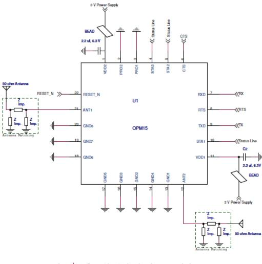
1.  $\perp$  = Connection to low impedance ground plane
