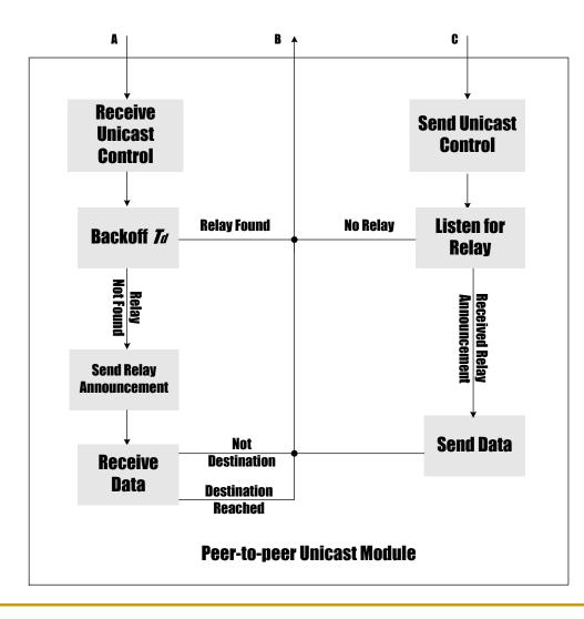
The unicast wireless link elects a relay wireless node for transmitting the data.
